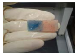
Figure 1 (left). Section of pig skin partially treated with NIMBUDERM™ (left half) after rinsing followed by saturation with Bromothymol blue dye solution. Blue area represents coverage of the treatment due to the electrostatic interactions between the dye and NIMBUDERM™.
